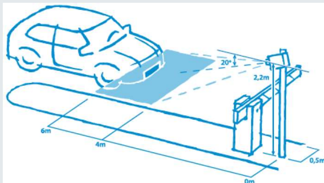
Figure 4: Behind the barrier mounting (ANPR Access HD)
