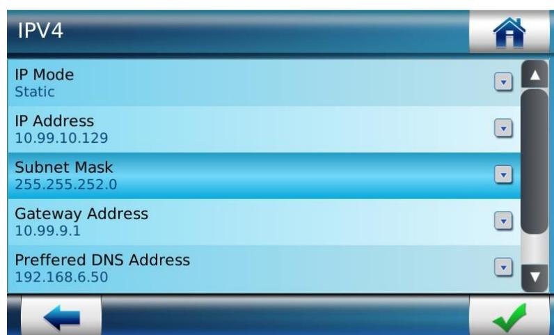
Figure 179: Configuring IP Address under Static IP Mode
