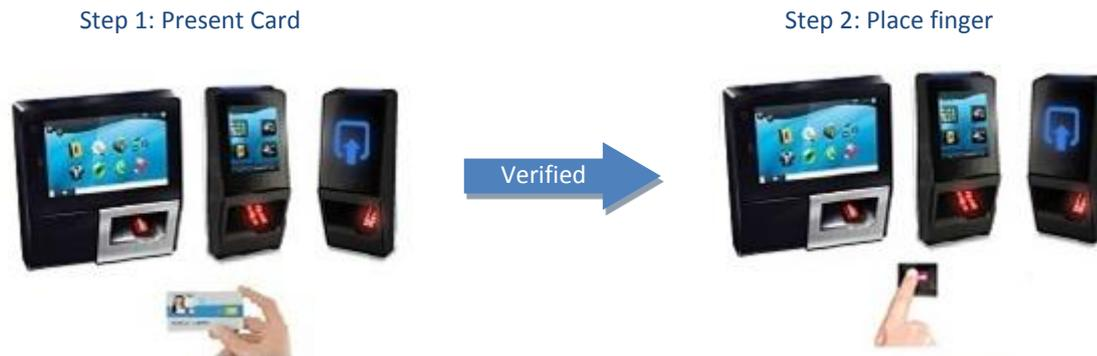
**Figure 333: Authentication with user's fingerprints on contactless card**
