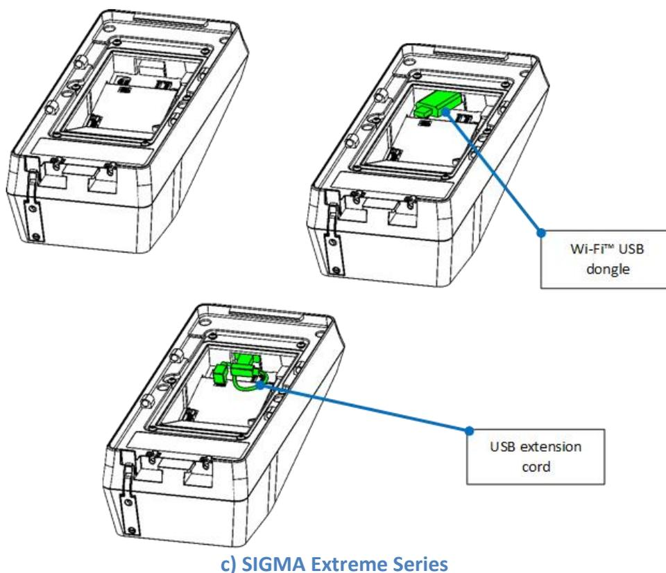
**Figure 5: MorphoAccess® SIGMA Family Series, MorphoWave® Compact terminal USB port with a Wi-Fi™ adapter**
