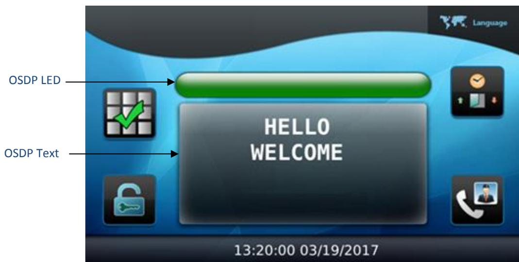
**Figure 359: OSDP LED and TEXT Screen on MorphoAccess® SIGMA terminal**
