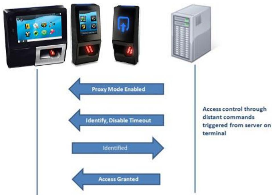
Figure 363: PROXY sample with a remote Identification process
