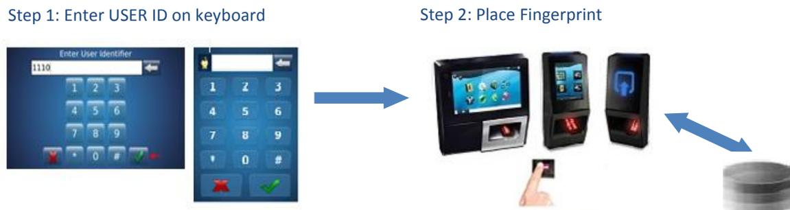
**Figure 337: Authentication with User ID entered from Keyboard and biometric check**
