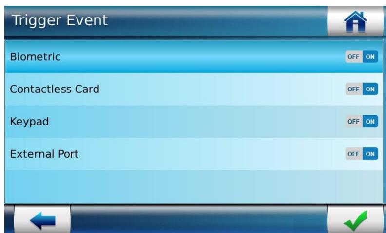
**Figure 190: Configuring the events on which authentication/identification is triggered**
