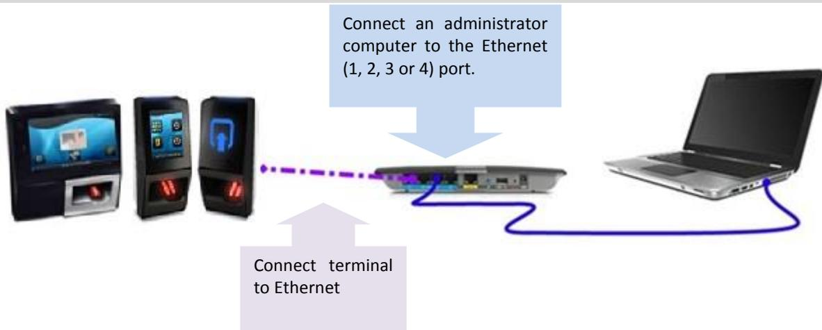
Figure 3: Connection through an Ethernet switch
