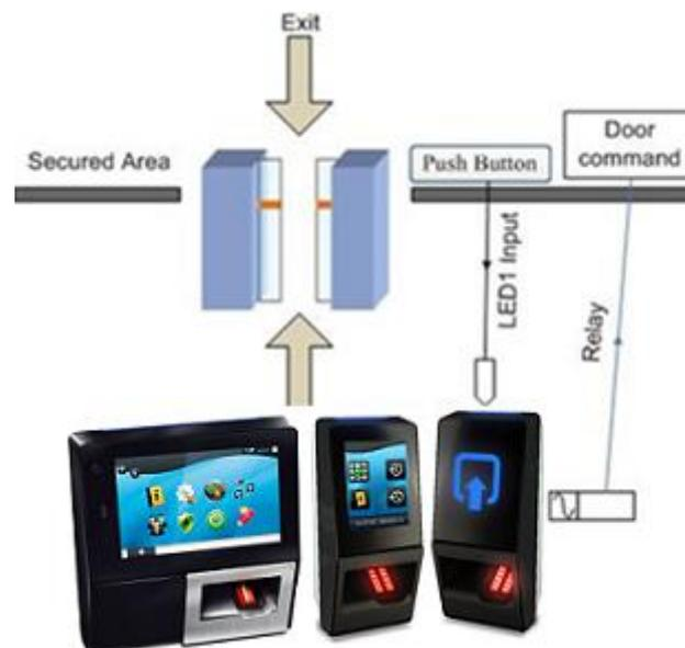
Figure 365: Internal relay activated by LED 1 signal
