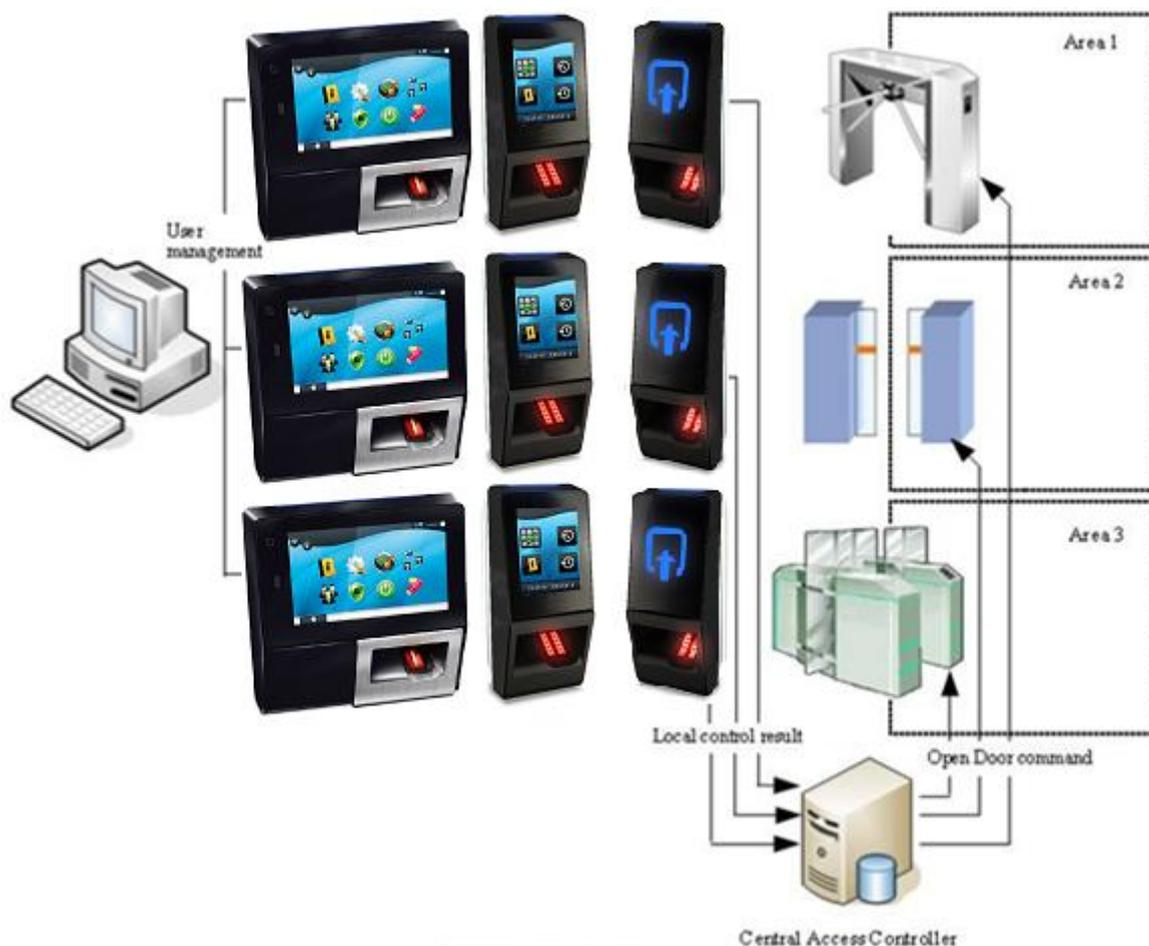
Figure 326: Typical access control system architecture for MorphoAccess® SIGMA Family Series, MorphoWave® Compact
