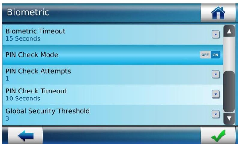
Figure 195: Setting PIN Check Mode
