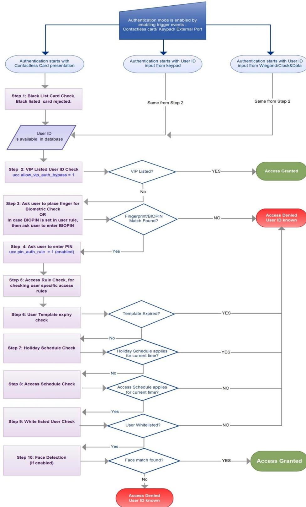
Figure 328: Access Control Flow Diagram in Authentication Mode
