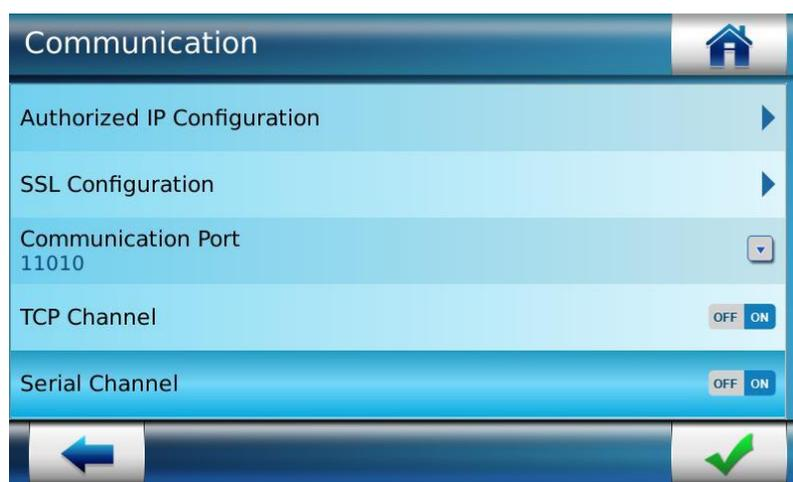
Figure 216: Enabling/Disabling RS422/RS485 Serial Channel
