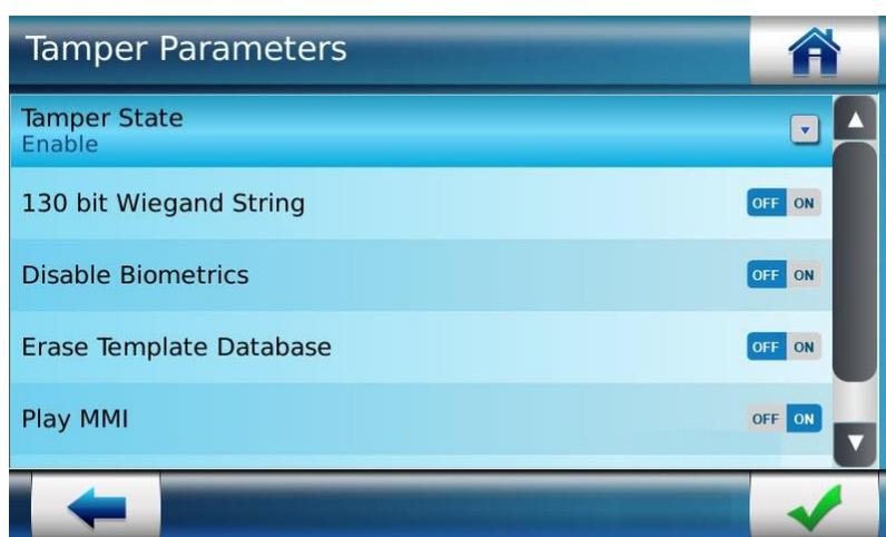
Figure 148: Tamper Parameters Configuration
