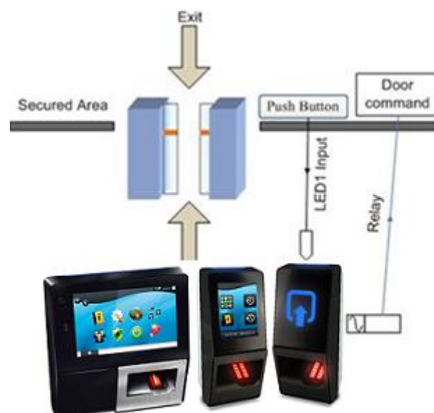
Figure 370: Internal relay activated by LED 1 signal
