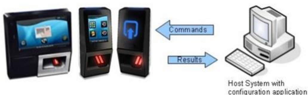
Figure 5: Configuration of a MorphoAccess® SIGMA Family terminal by a Host System
