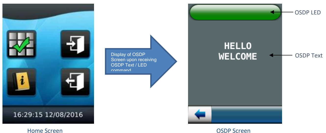
Figure 365: OSDP LED and TEXT Screen on MorphoAccess® Lite+ terminal
