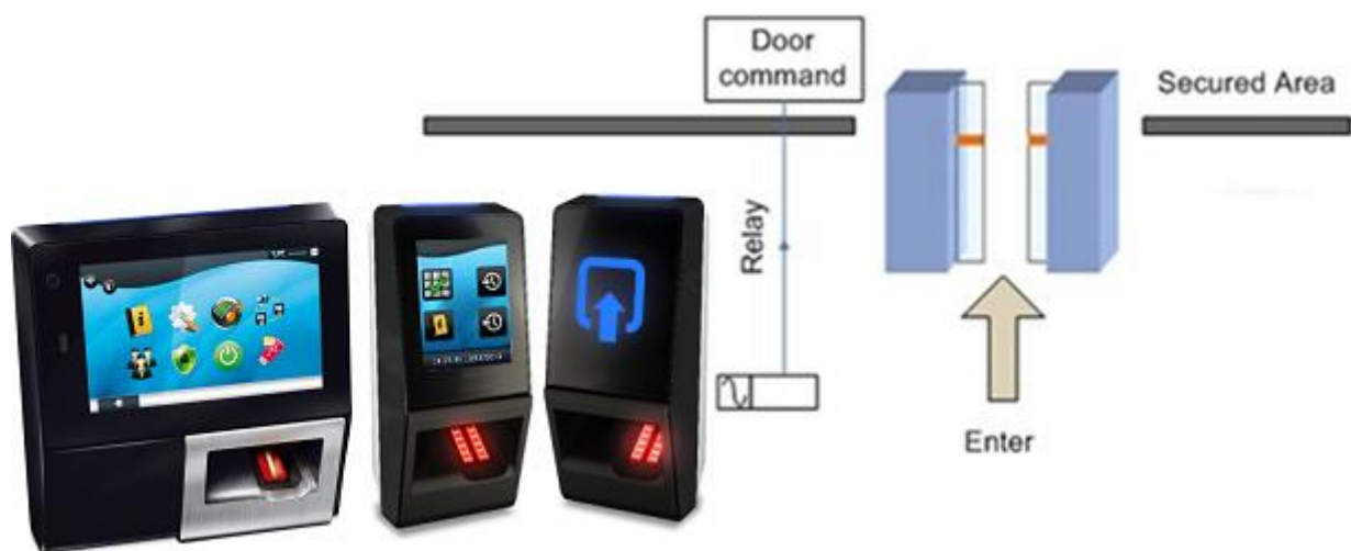
Figure 369: Using the internal relay on the Access and Time Biometric Terminal
