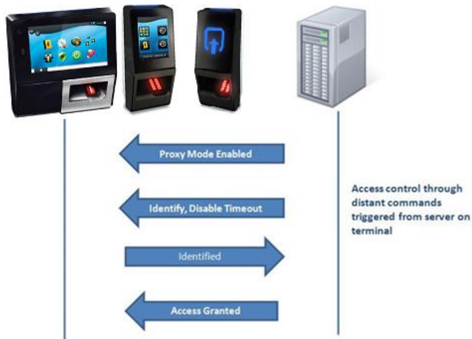
Figure 368: Distant commands sample with a remote Identification process
