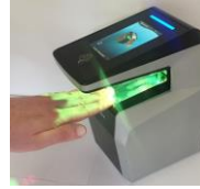
Do not place your hand on the edge of the optical sensor
