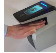
Do not place your hand too far up on the optical sensor
