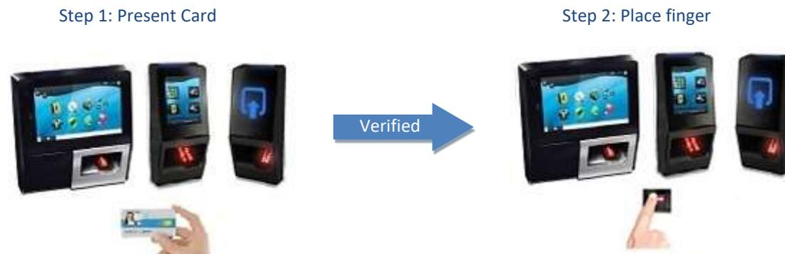
**Figure 332: Authentication with user's fingerprints on contactless card**
