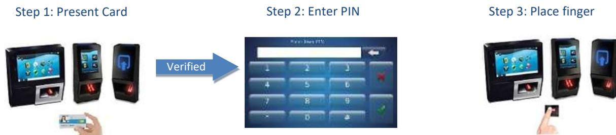
**Figure 333: Authentication with user's PIN Code and fingerprints on contactless card**
