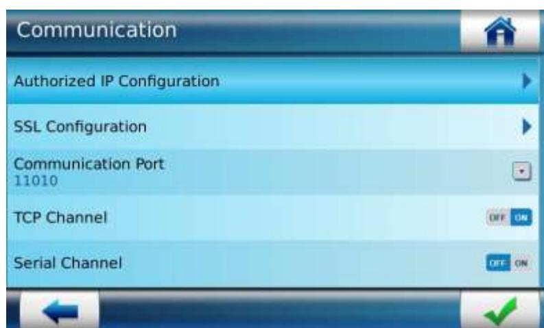
Figure 199: Authorized IP addresses Configuration
