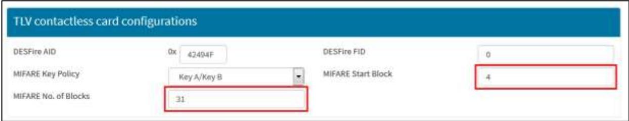
The screenshot displays the 'TLV contactless card configurations' web page. It features several configuration fields: 'DESFire AID' with the value '0x 42404F', 'DESFire FID' with the value '0', 'MIFARE Key Policy' with a dropdown menu set to 'Key A/Key B', 'MIFARE Start Block' with the value '4', and 'MIFARE No. of Blocks' with the value '31'. The 'MIFARE Start Block' and 'MIFARE No. of Blocks' input fields are highlighted with red rectangular boxes.
