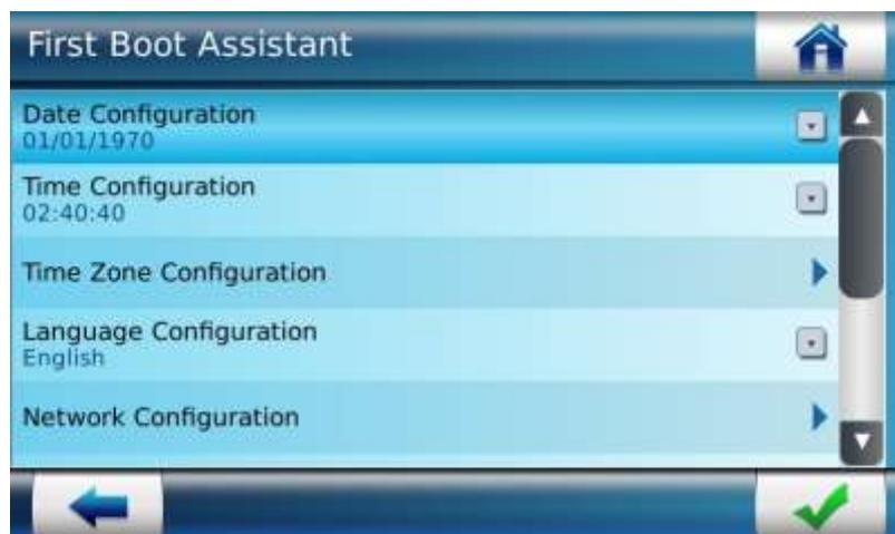
Figure 10: First Boot Assistant Screen displayed on Installation
