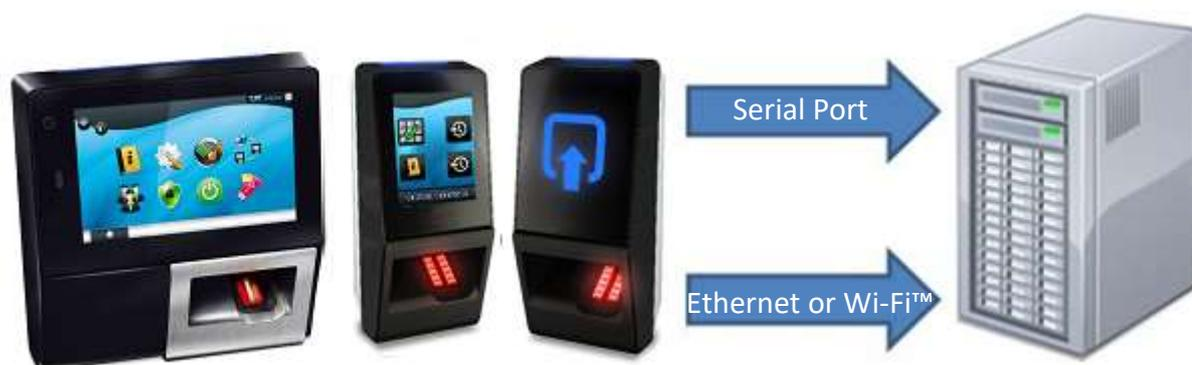
Figure 365: Sending access control result message to a distant system
