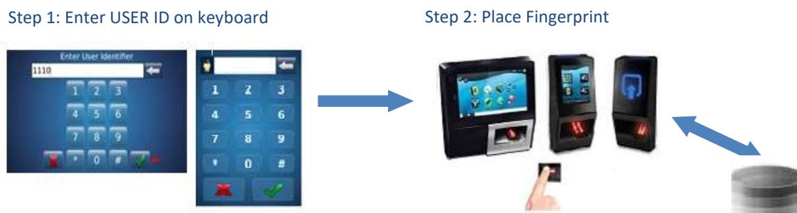
Figure 336: Authentication with User ID entered from Keyboard and biometric check
