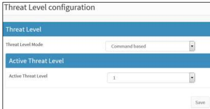
The screenshot shows a web-based configuration interface for threat levels. It has a title bar 'Threat Level configuration'. Below it, there are two main sections. The first section, 'Threat Level', contains a label 'Threat Level Mode:' followed by a dropdown menu currently showing 'Command based'. The second section, 'Active Threat Level', contains a label 'Active Threat Level' followed by a dropdown menu currently showing '1'. At the bottom right of the form, there is a 'Save' button.
