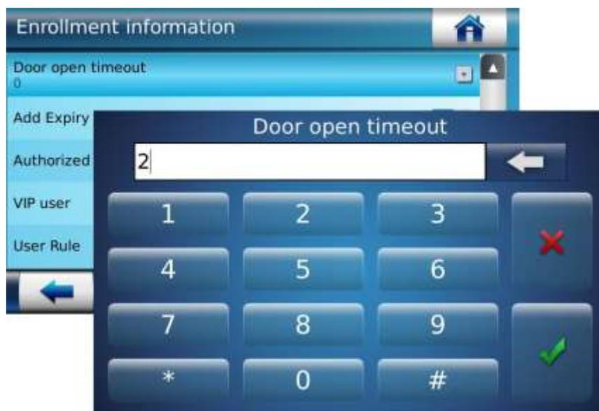
Figure 62: Configuring Door Open Time Out
