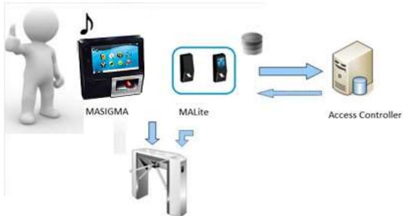
Figure 328: Access Granted Diagram for MorphoAccess® SIGMA Family Series, MorphoWave® Compact
