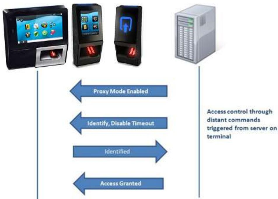
Figure 362: Distant commands sample with a remote Identification process
