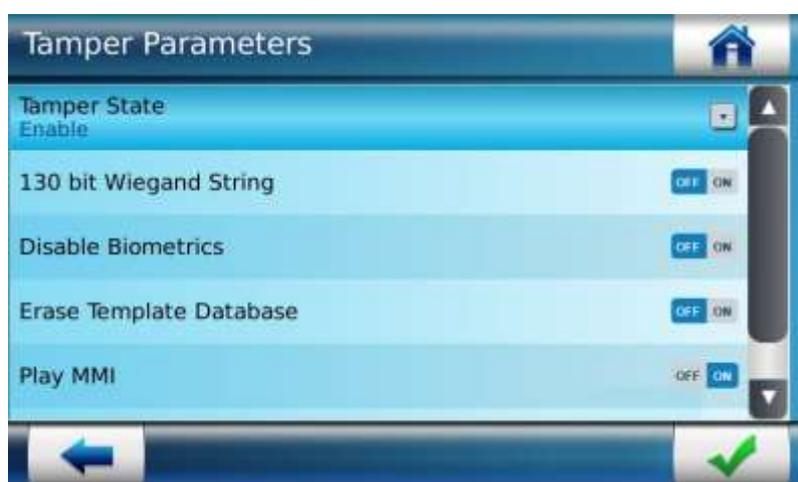
Figure 147: Tamper Parameters Configuration
