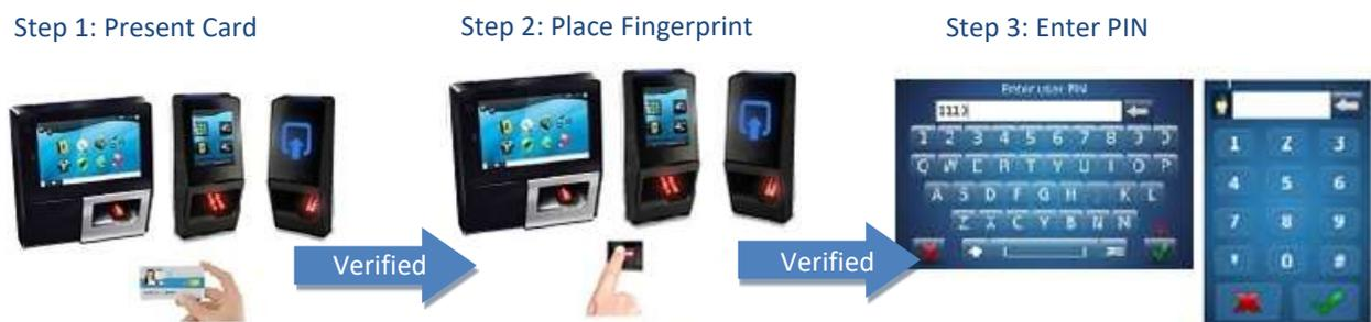
Figure 339: Authentication process specified by user's card
