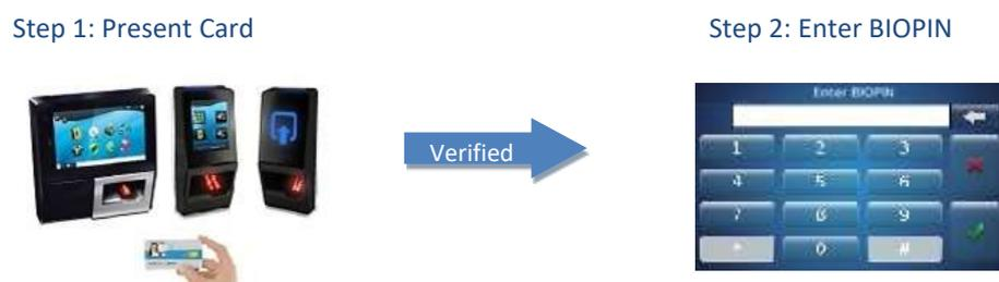
**Figure 334: Authentication with user's BIOPIN on contactless card**
