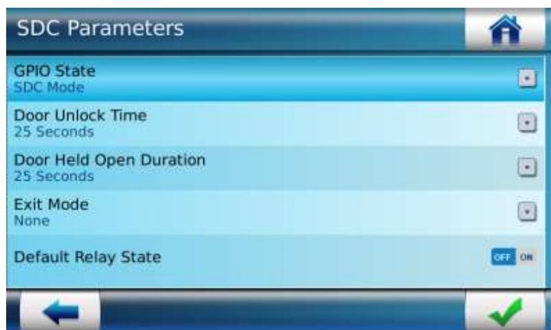
Figure 143: Configuring Parameters in “SDC Mode”
