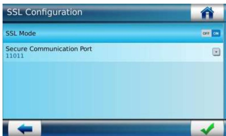
Figure 210: Configuring SSL Mode and parameters
