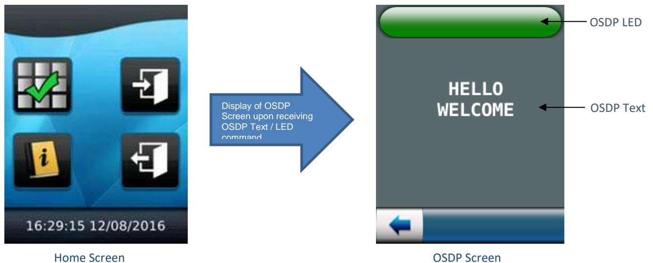
**Figure 359: OSDP LED and TEXT Screen on MorphoAccess® Lite+ terminal**
