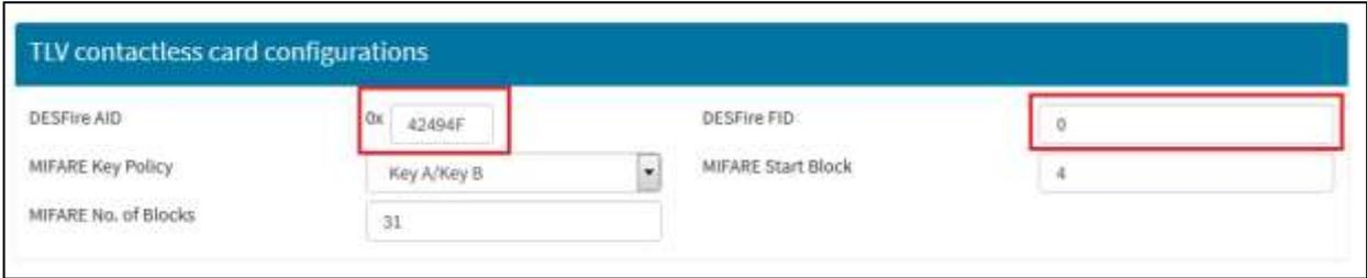
The screenshot displays the 'TLV contactless card configurations' web page. It features several input fields: 'DESFire AID' with the value '0x 42494F', 'DESFire FID' with the value '0', 'MIFARE Key Policy' with a dropdown menu set to 'Key A/Key B', 'MIFARE Start Block' with the value '4', and 'MIFARE No. of Blocks' with the value '31'. Red boxes highlight the 'DESFire AID' and 'DESFire FID' fields.
