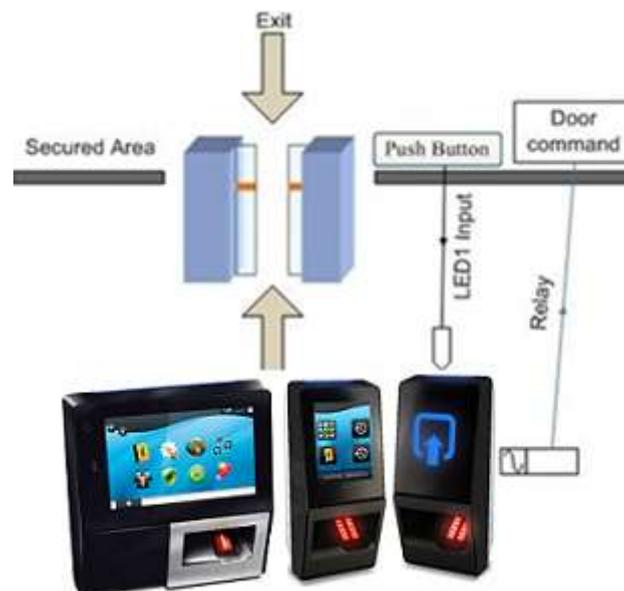
Figure 364: Internal relay activated by LED 1 signal
