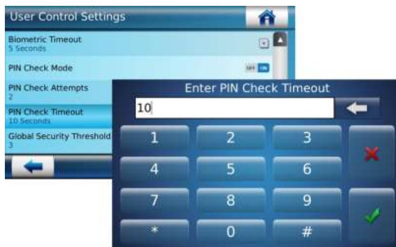
Figure 196: Setting PIN Check Timeout
