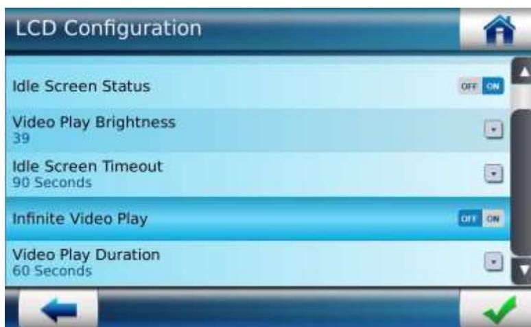
Figure 154: Infinite Video Play on idle screen
